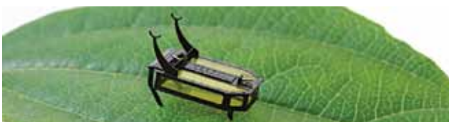
Look ma, no wires! A robotic beetle, which weighs about as much as three grains of rice, crawls, carries and climbs without being tethered to a power source (Credit: X. Yang, L. Chang, N.O. Pérez-Arancibia/Sci. Robotics 2020)
