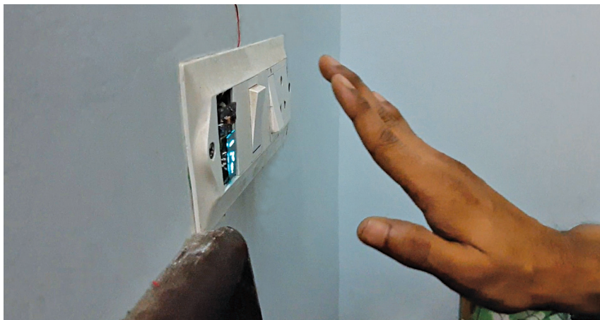
Fig. 9: Moving hand up in front of the contactless switch switches on light bulb
